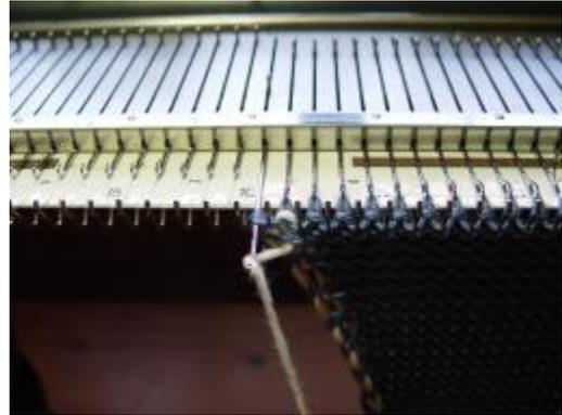
... and pull the 2<sup>nd</sup> needle to hold position.
