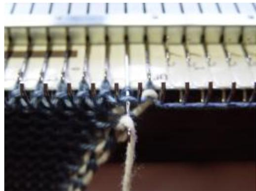
... and pull the edge needle to hold position. Note how the tuck stitch on the 2<sup>nd</sup> needle dropped off to form a purl-wise slip.
