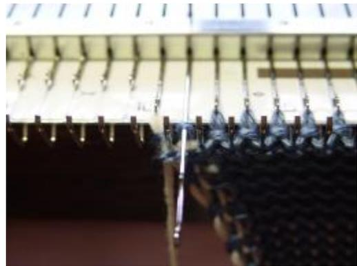
Use the other extra length of yarn to wrap the 2<sup>nd</sup> needle from the edge on the carriage side; again, the yarn passes over the needle toward the carriage. Manually knit this needle...
