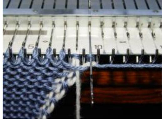
After knitting the row – in this case, from right to left – the HP needles contain floats and the manually knit needles contain stitches knit with the main yarn.
