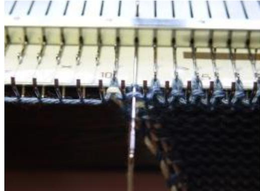
Now, knit the extra yarns and position the needles for the next pass of the carriage from left to right.
